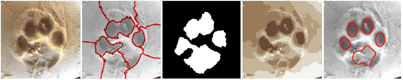
Fig. 3. Segmentation of footprint by traditional algorithms (from left to right): Input color image, Normalized Cuts [8], Graph Cuts [9], KM [10], and DRLSE [11] results. Similar results are observed for depth images.
